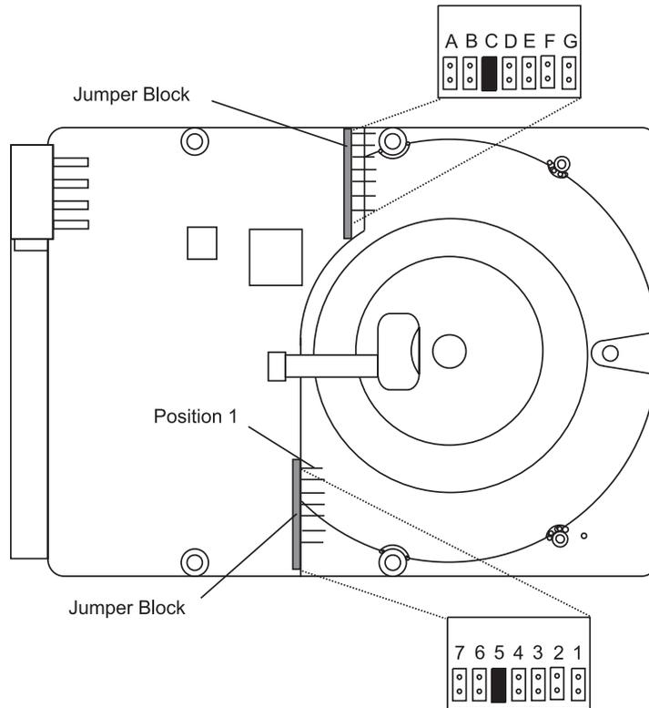
The previous illustration shows the pin positions on the 9.1 and 18.2GB Ultra SCSI disk drives.
