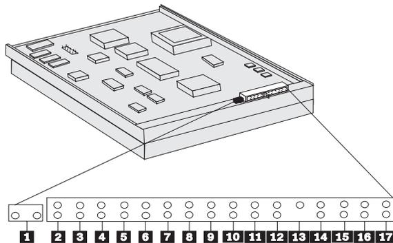
The jumper block on the drive has 16 pin positions (2 through 17). Term Power Enable (1) is located to the left of the jumper block. Refer to the previous illustration.
