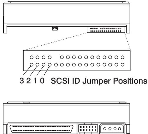
The previous illustration shows the pin positions on the 9.1 and 18.2GB Ultra SCSI 1" high disk drives.
