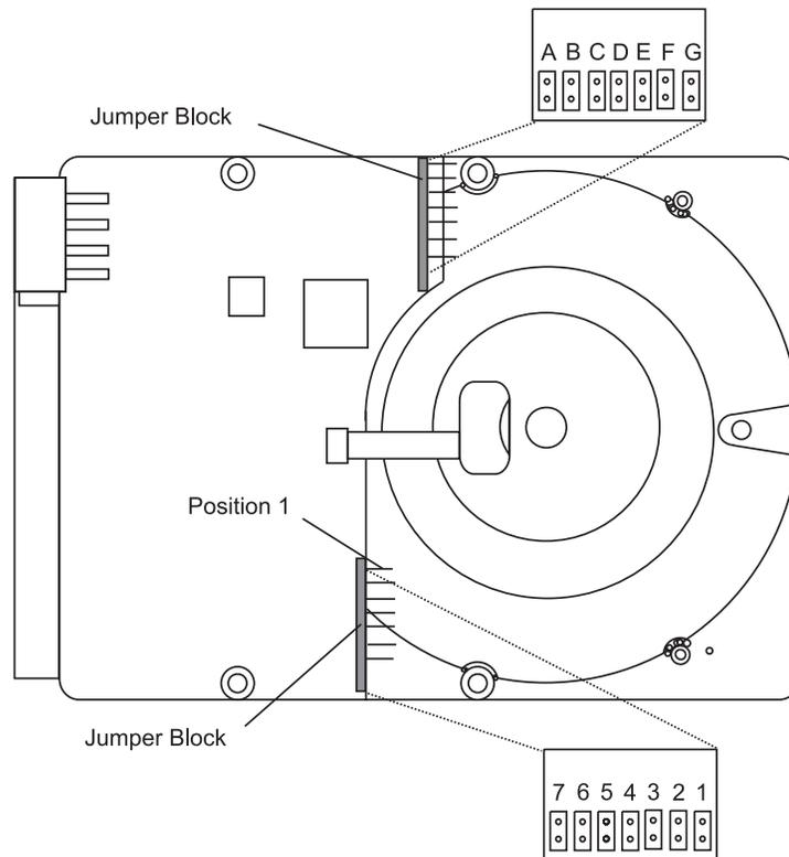
The previous illustration shows the pin positions on the 9.1, 18.2, and 36.4GB Ultra SCSI disk drives, no jumpers are required.
