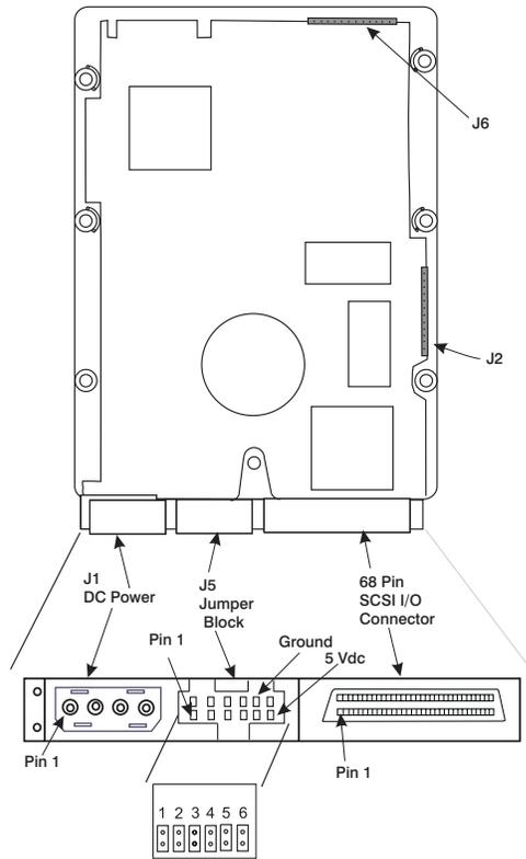
The previous illustration shows the pin positions on the 9.1, 18.2, 36.4, and 73.4GB Ultra SCSI disk drives, no jumpers are required.
